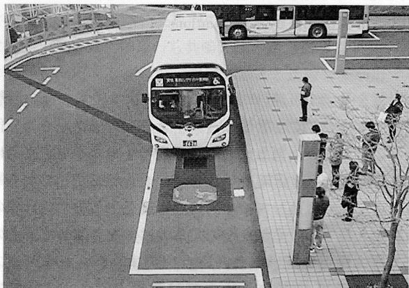
Fig. 16 IPS hybrid bus at bus stop at Big Site, Tokyo.
