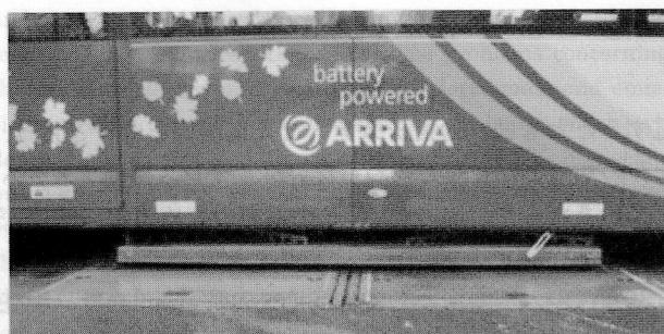
Fig. 5 Secondary coil taken down on primary coil.
