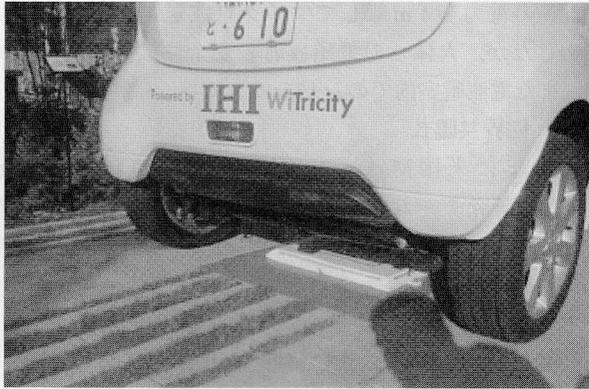
Fig. 10 Magnetic-resonance system of wireless power transfer.
