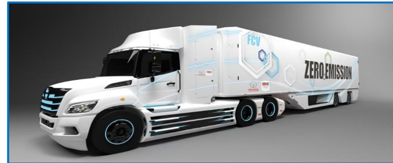
HD FC truck based on Hino XL series for the US market, using Mirai’s stacks. The road test was conducted in 2021.
