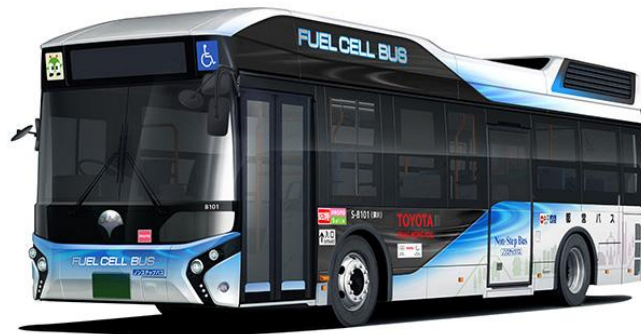
FC bus, “Sora” launched in Tokyo, in 2017, Feb., using two Mirai’s FC stacks, Drive range: about 200 km
