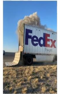
EV Battery pack in trailer in TX, Mar 2023
